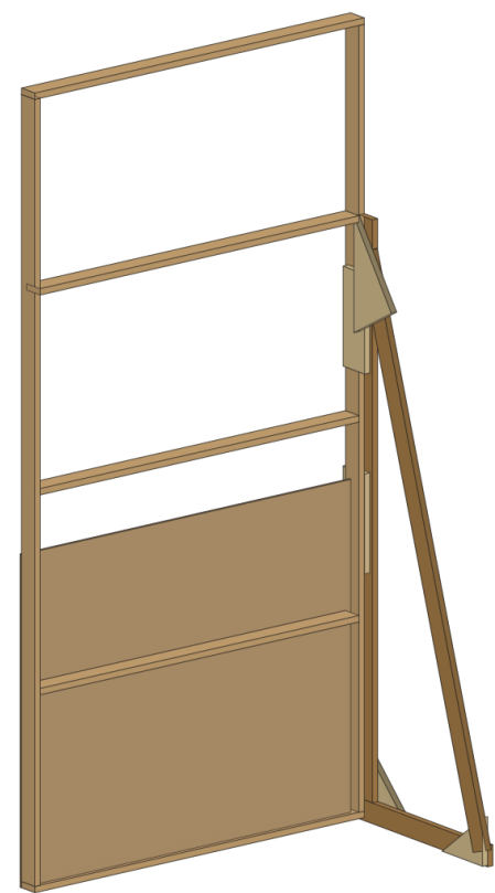
Flat from upstage, skin shown on the lower 40" only, with its jack.
